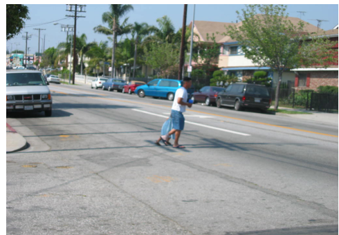
Boyle Avenue's wide streets pose a danger to pedestrians. Street design standards in other cities allow for narrower lanes on roads with 45 mph or lower speed limit.
